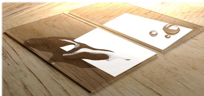
Figure 2: Illustration of contact-angle on glass surface without (left) and with (right) the application of the SurAChem® HP 310
