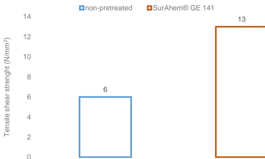
**Grafik 1:** Increase of the tensile shear strength by the application of the SurAChem<sup>®</sup> GE 141 adhesion promoter on PPS/sandblasted stainless steel.
